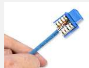
Keystone jacks are smaller connectors used for terminating individual cables . Fit into wall plates , floor boxes, and patch panels.
